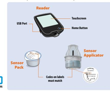
1 Assemble and Apply Sensor to your body
