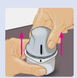
Lift Sensor Applicator out of Sensor Pack.
