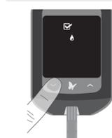
3. Press and hold the down arrow for 3 seconds to mark the test as a control solution test. The appears. The meter is now ready for you to apply control solution to the test strip.
