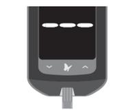
5. Hold the control solution to the test strip until: You see 3 short lines on the meter screen. This means you have applied enough control solution and the meter is reading the control solution.
