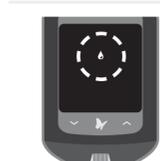
The blinks, indicating the meter is ready for you to apply a sample to the test strip.
