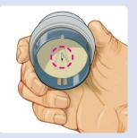
Sensor Applicator is ready to apply Sensor.
